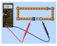
We can measure voltage differences with a **voltmeter** (as shown on the left). The voltmeter has a black and a red lead. To find out the voltage difference between two points on a circuit, put one lead on one point and the other lead on the other point. The voltmeter cannot be part of the circuit for it to work. **4.** In CCK, set up a circuit that has one light bulb and one battery. Measure and record the current going into the light bulb and the current coming out of the light bulb.
